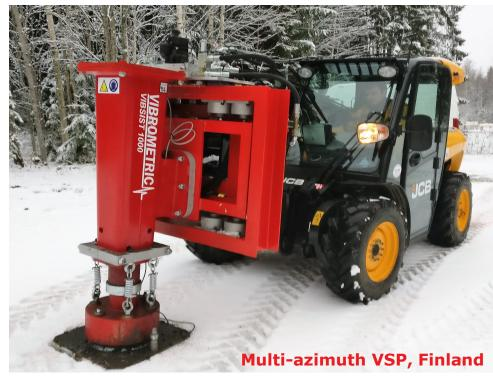
The VIBSIST-1000 is a **safe, non-destructive and environmentally friendly high-resolution seismic source**. It is **specially designed for use in forest areas**, so that cutting trees can be avoided.
