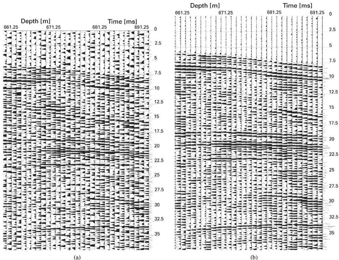
Fig. 9. Source gather measured with the PH70 SIST piezoelectric source. (a) Portion of the long SIST sequence. (b) Decoded profile (5–40 Hz, 10 s sweep, 200 impacts).
