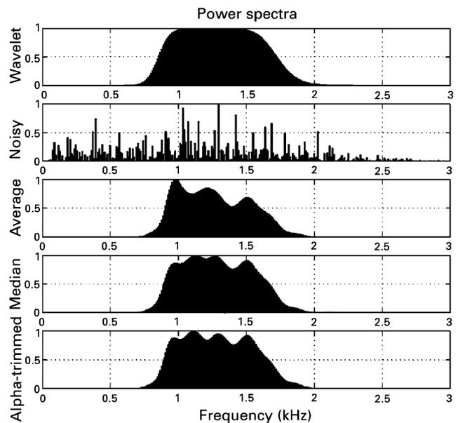
Fig. 4. Power spectra of the corresponding time domain signals of Fig. 3. Clearly, the median techniques are better than the straight sum.
