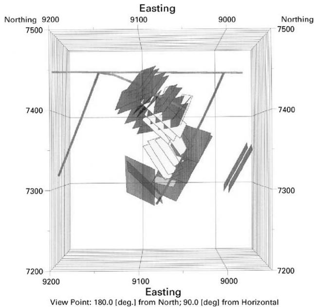
Fig. 10. Structural model of the investigation site at GTS as inferred from the SIST tunnel-to-hole and crosshole investigations.
