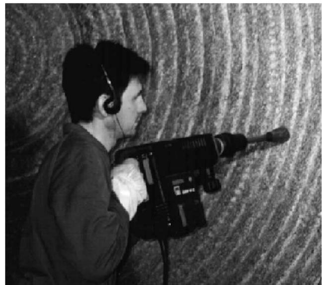
Fig. 6. SIST tunnel-wall source built starting from an electric demolition hammer.
