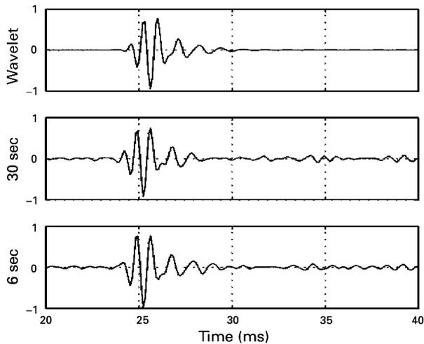
Fig. 2. The synthetic model (above) and the decoded signals corresponding to a 30 s, 18–30 Hz sweep (middle) and to a 6 s, 90–150 Hz sweep (below).
