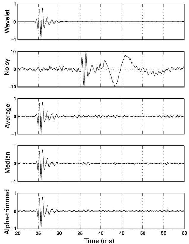
Fig. 3. Different techniques of extracting the useful signal from a noisy coded sequence (denoted “noisy”).
