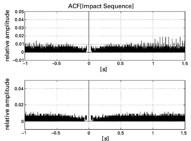
Fig. 1. Auto-correlation functions of the linear frequency (above) and the linear period (below) time coding schemes. The zero-lag peak in both cases is normalized to one and only a part of it is shown. The linear period scheme displays less spurious spikes. The spikier the  $ACF\{\psi(t)\}$ , in Eq. (2), the more correlation noise in the reconstructed  $r_d(t)$ .
