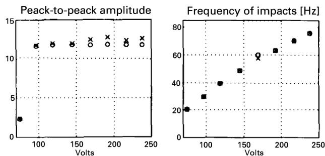
Fig. 5. Variation of the peak-to-peak amplitude and impact frequency with the input voltage, determined experimentally for an electric hammer drill.
