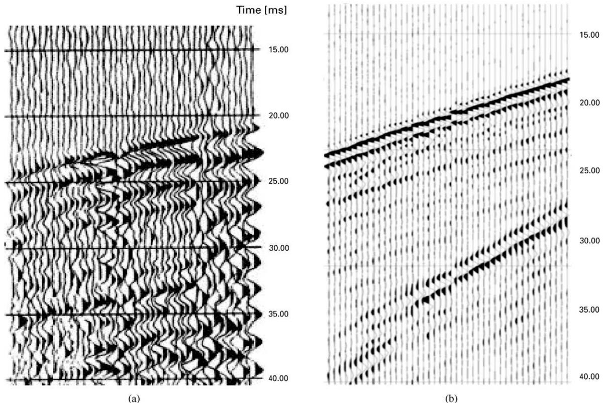
Fig. 8. Axial component receiver gathers obtained at GTS from a single-pulse source (PH52) (a) and the SIST20 source (b) (18–30 Hz, 20 s sweep, 500 impacts).
