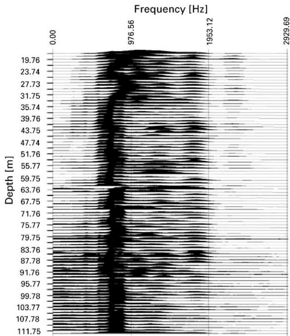
Fig. 7. Amplitude spectra of a Z-component VSP profile at GTS. A part of this profile is shown in time domain in Fig. 9(b). The signature of the SIST source from Fig. 6, used to survey this profile, extends from 500 Hz to beyond 2 kHz. The highly attenuative rockmass at GTS absorbs most of the frequencies above 1 kHz.
