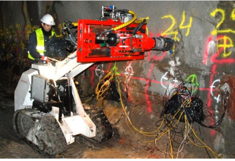
The VIBSIST-200 is an environmentally friendly seismic source. This a non-destructive alternative that does not create environmental pollution such as chemicals, sound, etc. Legal risks frequently associated with using explosives are eliminated.
