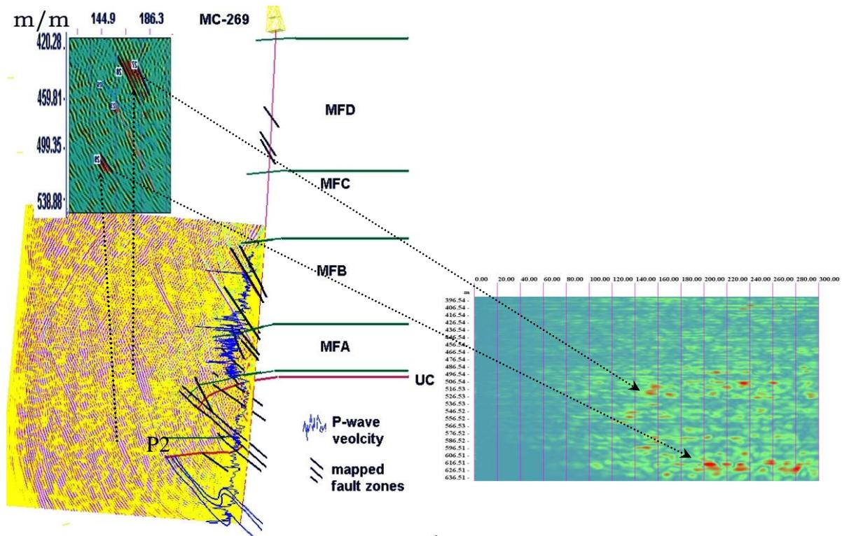
Figure 4. Downhole seismic images from drill hole MC-269 showing defined faults, notably the P2 and related structures (left) and the enveloped point-diffractor processed profile (right). The two features marked with arrows indicate two coherent reflections and diffraction anomalies at depths corresponding to the upper and lower unconformity surfaces at the P2 fault.
