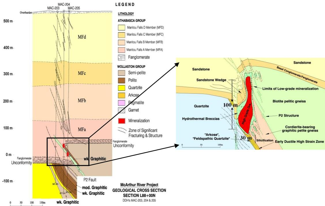
Single-hole measurements were done using a water-coupled SPH54 piezoelectric source with 1 kHz center frequency in borehole MC-269 and with 2 kHz center frequency in borehole MAC-204. The MC-269 section was measured from 306m to 571m and the section in MAC-204 from 257m to 571m.
