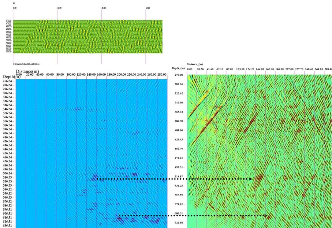
Figure 3. Borehole MC-269. Example of shotgather (upper left), stacked profile with enhanced point diffractors (left) and stacked profile with enhanced steeply dipping reflectors (right).
