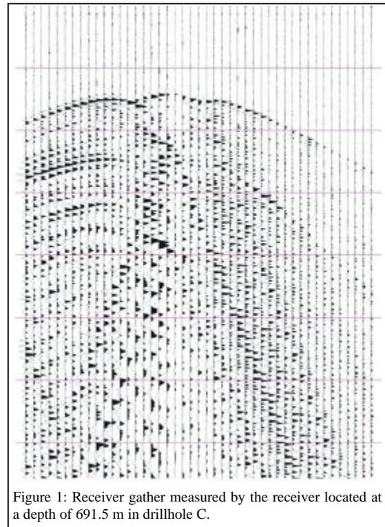
Figure 1: Receiver gather measured by the receiver located at a depth of 691.5 m in drillhole C.
