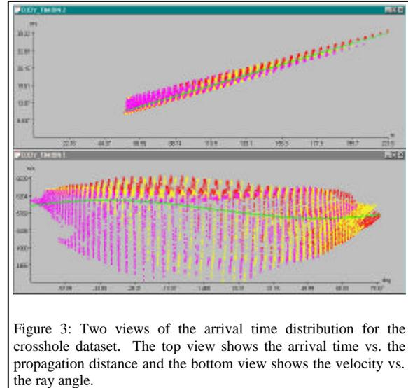
Figure 3: Two views of the arrival time distribution for the crosshole dataset. The top view shows the arrival time vs. the propagation distance and the bottom view shows the velocity vs. the ray angle.
