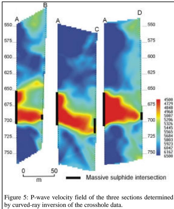
Figure 5: P-wave velocity field of the three sections determined by curved-ray inversion of the crosshole data.
