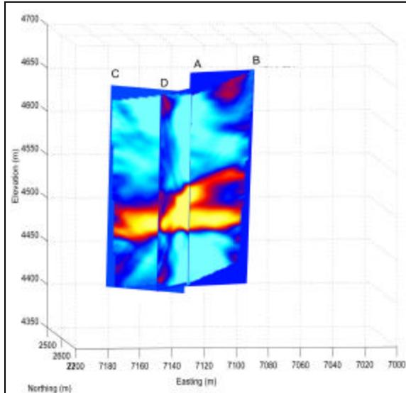
Figure 4: 3-D view of the velocity maps from the three crosshole sections.
