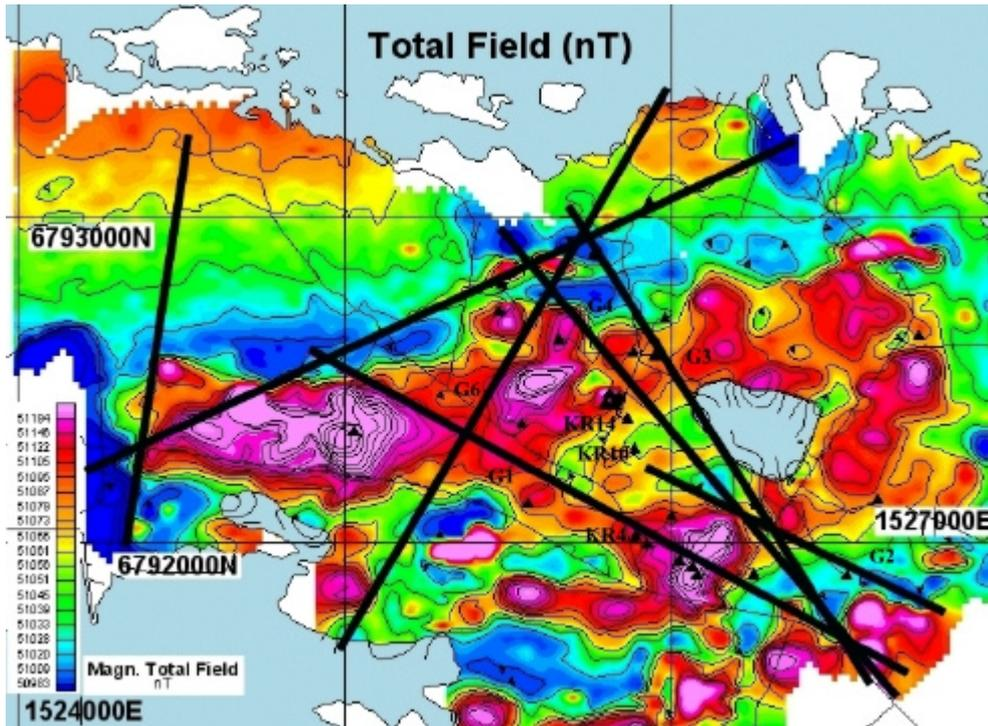
*Figure 1.* Magnetic map of the Olkiluoto area. Map contains interpretations based on visual assessment of the data (black lines). Definition of their absolute locations would require model calculations. Black triangles show the locations of the drilled holes.
