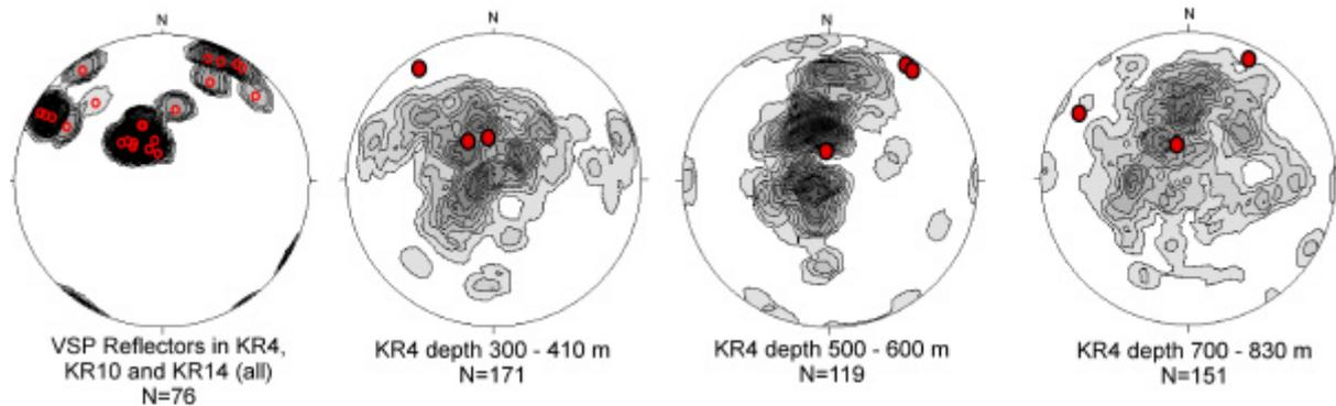
*Figure 4.* The VSP reflectors of KR4, KR10 and KR14 (all, on the left those found from KR4 are denoted with red dots) and the fracture orientation of KR4 short sections A (300-410 m), B (500-600 m) and C (700-830 m) with reflector orientations from same depth level. Lower hemisphere, area-equal projection.
