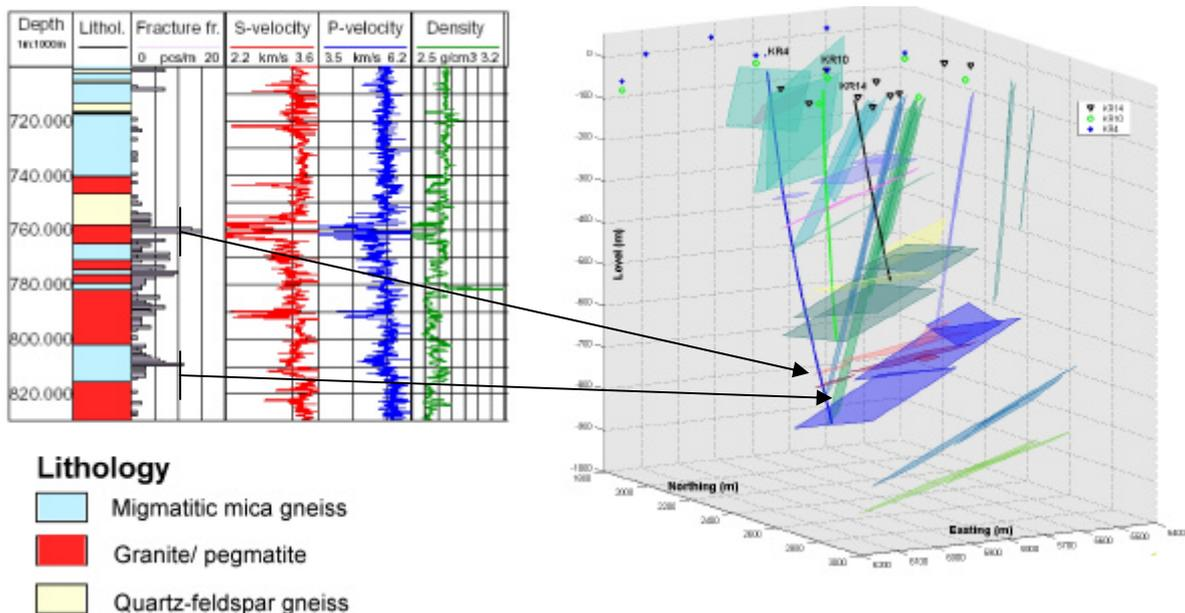
Figure 3. Site scale presentation of the VSP reflectors from boreholes KR4, KR10 and KR14, and an example of lithologies, fracture frequency and sonic and density logs from KR4 depth level 700-780 m (a gently dipping reflector 760 m, a sub-vertical 810 m, and location shown with an arrow).
