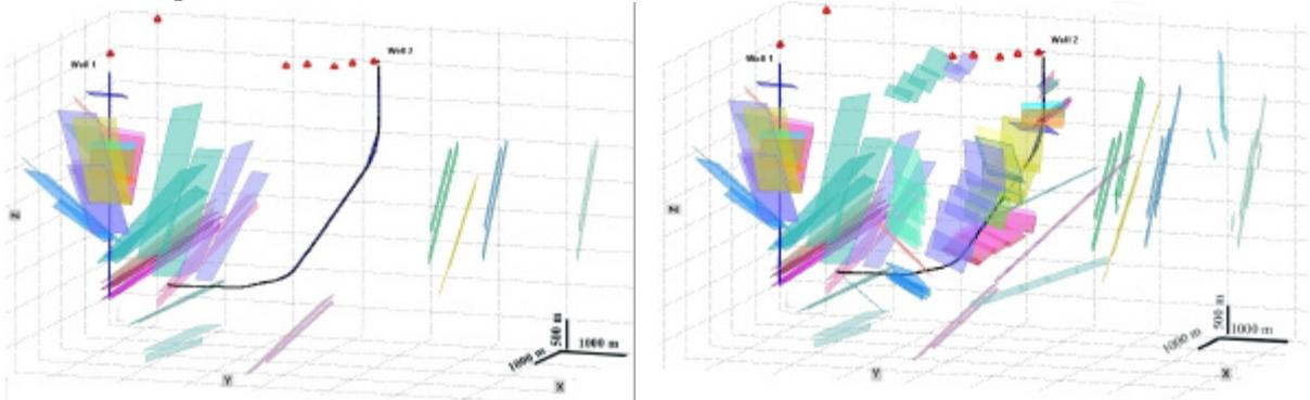
*Figure 4.* 3D view of interpreted reflectors. (a) Left: one option for elements identified from Well 1 only; (b) Right: elements identified from both Well 1 and Well 2.
