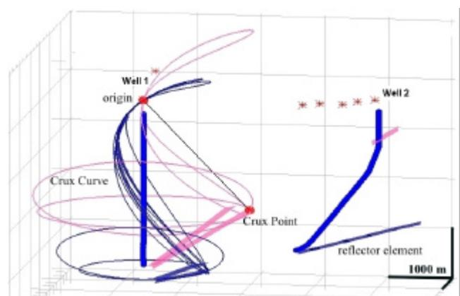
*Figure 3.* Crux Point diagram for both wells. The Crux Point curves and the interpreted reflecting elements of the two gently dipping reflectors marked in *Figure 2* are represented in 3D.
