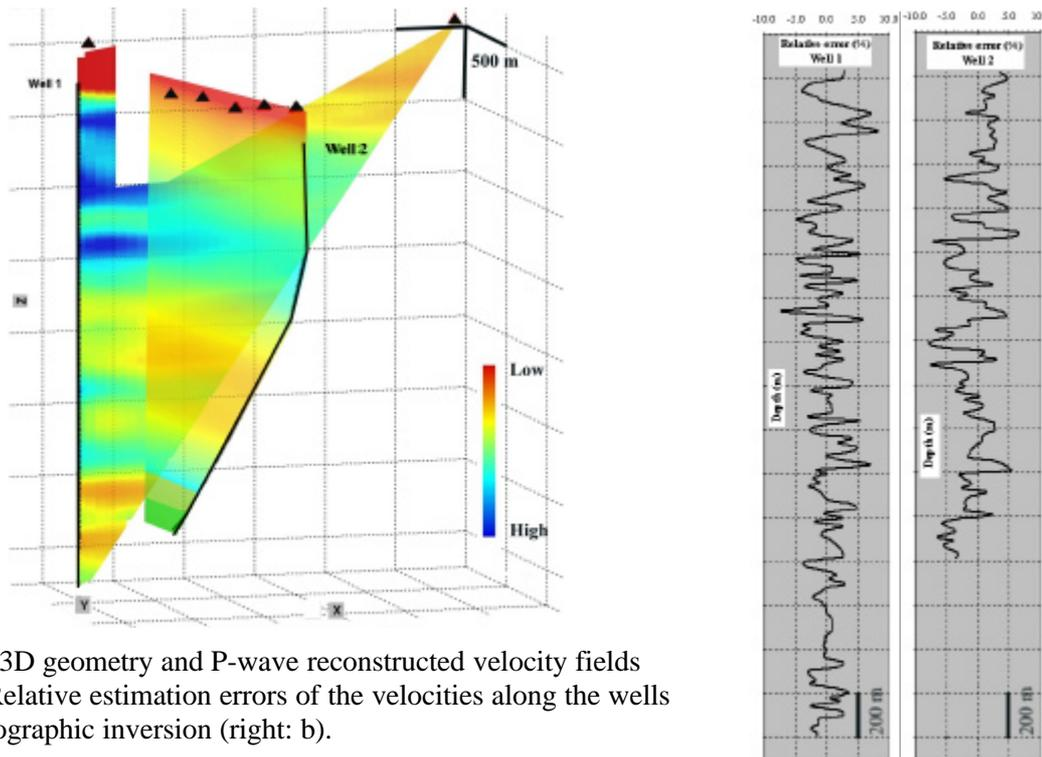
*Figure 1.* 3D geometry and P-wave reconstructed velocity fields (left: a). Relative estimation errors of the velocities along the wells from tomographic inversion (right: b).
