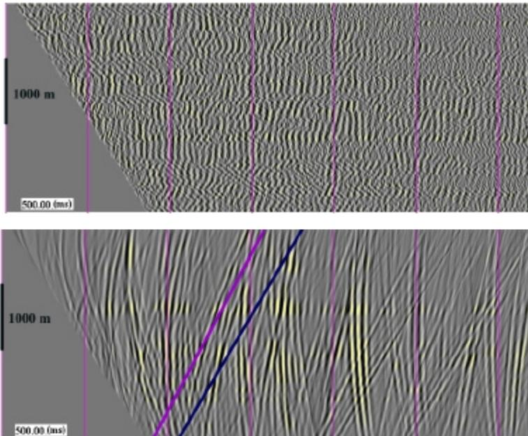
*Figure 2.* Axial zero offset VSP profile acquired from Well 1, after the Pre-Processing stage (above: a) and after the Reflector Imaging stage (image space & dip filtering) (below: b). The time curves generated by two gently dipping reflectors are marked.
