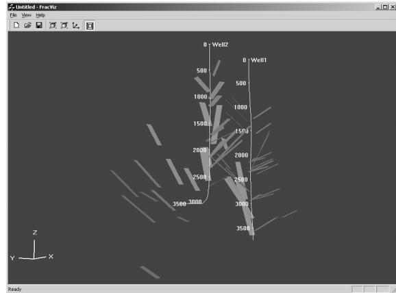
Figure 4. Visualisation of the interpreted reflector elements.
