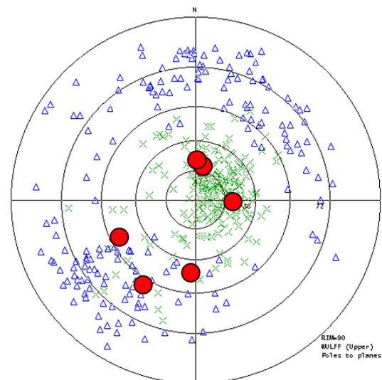
Figure 4: Stereonet comparing planes identified by VSP processing (large dots) and image log analysis (faults and fractures shown as open triangles, bedding planes as crosses) for the reservoir section in one of the study wells.
