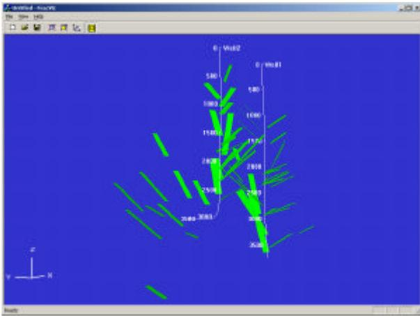
Figure 3: Visualisation of interpreted reflector elements.
