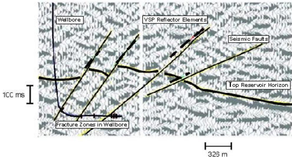
Figure 5: Seismic line through well showing how integration of seismic (solid lines), VSP (dashed lines) and well-derived information enables a well-constrained subsurface structural model to be produced.
