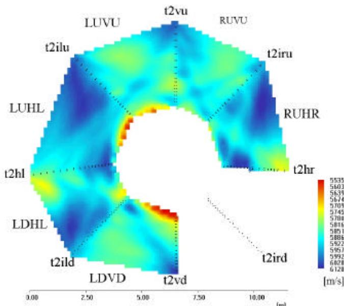
The six “normal sections” produce the tomogram from Figure 18. The velocity .vs. angle distribution is presented in Figure 19. In this case, the anisotropy is probably real. Its direction is exactly vertical and its magnitude is 2 %.
