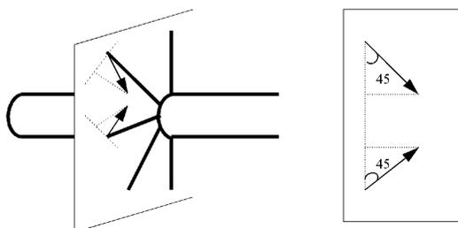
Figure 3. Orientation of the transmitter and receiver probes with respect to the tunnel and the plane of the boreholes.
