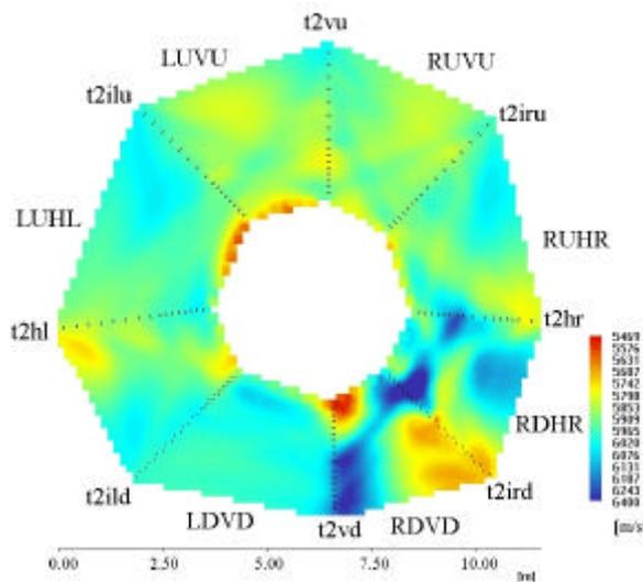
The tomographic section in Figure 14 was obtained with no corrections, except for the ones described in Sections 4.1 and 4.2. It is apparent that sections RDHR and RDVD have a pathologic appearance.
