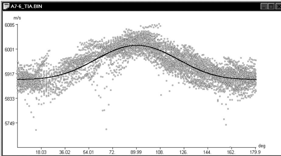
Figure 19. Velocity vs. Angle distribution for six sections. The number of data points is appr. 6000. The curve represents the least squares fit of an anisotropic model with three parameters. The best fit values are: maximum velocity (model) 6050 m/s, direction of maximum velocity - vertical, elliptical variation (period  $p$ ) 2%, secondary variation (period  $p/2$ ) 0.45 %.
