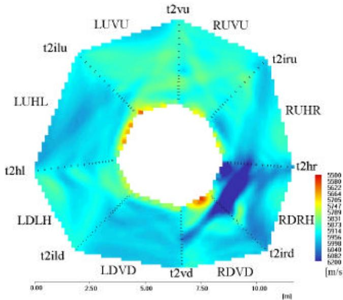
Figure 17. P-wave velocity of the eight crosshole sections of TBM round 2.
