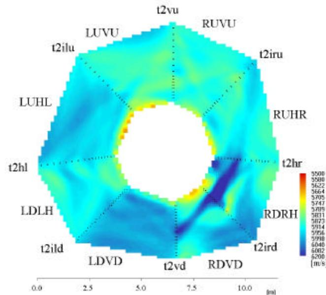
Figure 16. P-wave velocity of the eight crosshole sections of TBM round 2.
