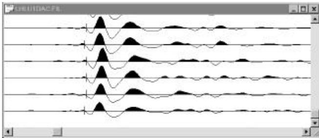
Figure 4. Part of the D&B LH-LU section bandpass filtered from 5 to 32 kHz.
