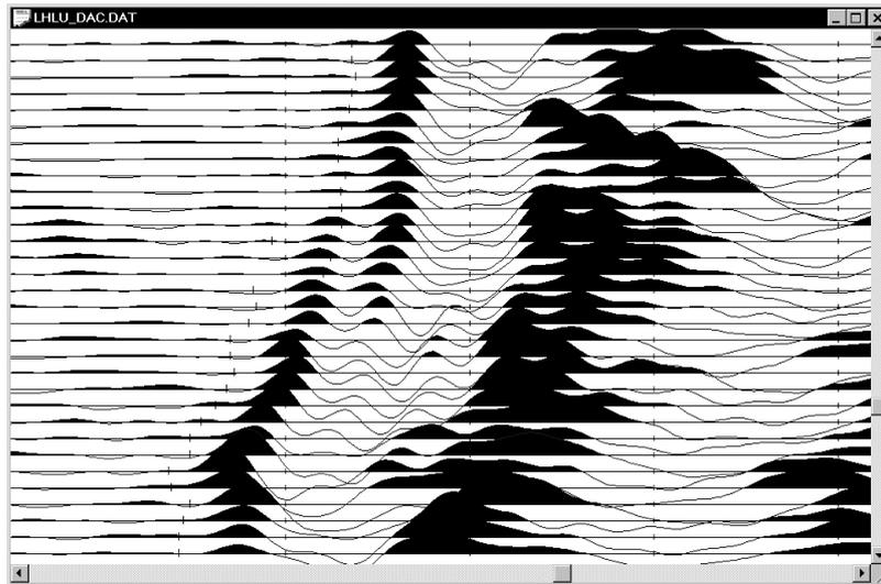
Figure 13. Part of the section LHLU, of D&B round 7, plotted with reduced velocity  $v=3450$  m/s. With this presentation, shear wave arrivals should be roughly vertical. One notes the double S-wave arrival, probably due to splitting. If due to anisotropy, the velocity ratio between SH and SV waves corresponding to such splitting is estimated to 1% or less.
