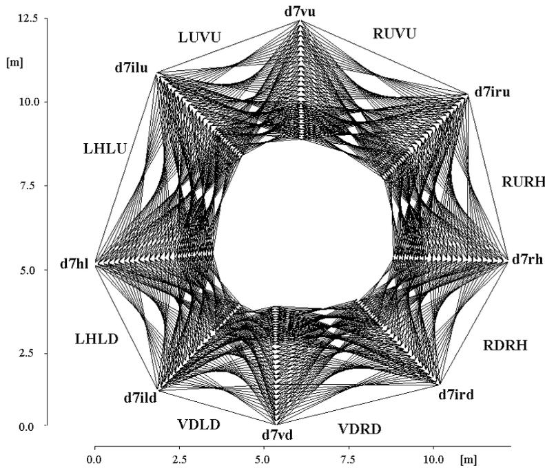
Figure 2. Ray diagram of the eight crosshole sections measured around the D&B tunnel. Every section is identified by the corresponding pair of boreholes. The first borehole in the name of the section is the source borehole. Similar coverage was achieved around the TBM tunnel (borehole names start with t2, instead of d7, in this case).
