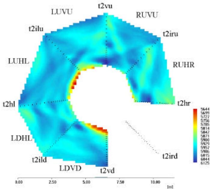
Figure 20. P-wave velocity of six crosshole sections of TBM round 2, after applying corrections. (Sections RDHR and RDVD were ignored.) The mean velocity is 5993 m/s and the residual mean square error after inversion was 1.21 ms. The inversion was done on 5995 travel times with 0.15 m X 0.15 m block size.
