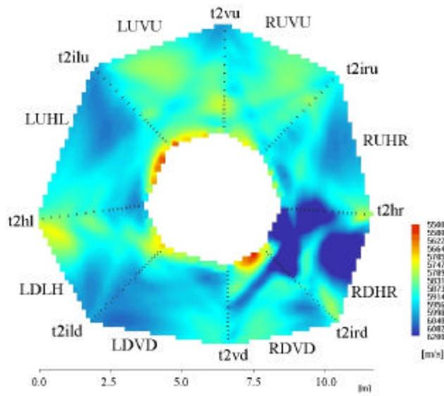
Figure 15. P-wave velocity of the eight crosshole sections of TBM round 2.
