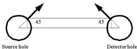
Figure 9. The true source - receiver distance is AB. The borehole coordinates give the segment OO'.
