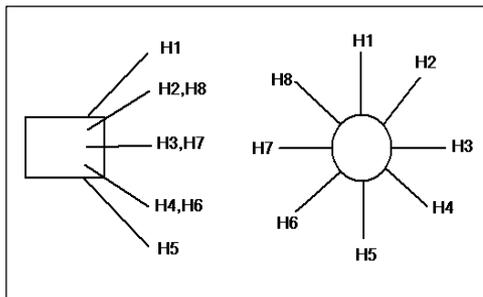
Figure 22. Suggested layouts of radial boreholes, to allow experiments to be conducted before and after the excavation of the following tunnel section.
